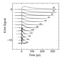
Fig. 1 Echo signals of CuCl quantum dots at various temperatures. The radius of the quantum dots is 3.1nm. The decay time becomes shorter with the temperature rise. Slow rise observed in the initial part come from the antihole structure in the persistent spectral hole burning.
