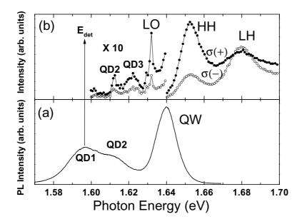
**Figure 1**. (a) Photoluminescence spectrum of GaAs quantum dots excited with a continuous wave Nd:YVO<sub>4</sub> laser. (b) Polarized photoluminescence excitation spectra. The detected energy position is set to the first excited state of the quantum dots, which is obtained from the PL measurement. The closed (open) circles show the same (opposite) circular polarization as the excitation laser
