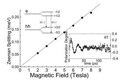
**Figure 4**. The observed Zeeman splitting (closed circles). The g-factor is 0.47. The inset shows degree of polarization obtained at 6 T (open circles). The solid curve is a fit. A scheme shows optical transition from Zeeman components of QD1 state.
