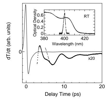
**Figure 1.** The results of pump-and-probe transmission measured by using delay time modulation. A clear damped oscillation is observed in the expanded plots. A dashed line represents the results of fitting by a damped cosine function. Inset : Absorption spectrum of CuBr QDs in glass at room temperature. Mean radius of the sample is 5.4 nm. A dashed line shows the spectrum of the pump and probe pulse.
