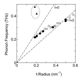
**Figure 3.** Size-dependence of the frequency of oscillatory component (solid circles). Dashed lines represent the size-dependence of the lowest l=0 mode and l=2 mode calculated by using elastic continuum model. Solid triangles represent the frequency of the high-frequency component (see text). Open circles show the results of PSHB spectroscopy. The data of two different measurements coincide quite well.
