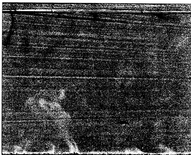
Fig.3 Ratio of Rhodamine B and Rhodamine 110 images. Black and white level corresponds to 0.95 and 1.05, respectively.
