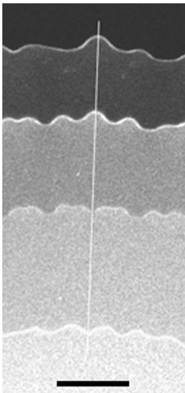
FIG. 21. Sequence of edges showing the whole process of formation of two peaks on each finger and the subsequent merging into three fingers. The time separation is  $\Delta t = 0.5$  ms with the first flash at 0.2 ms after contact. The scale bar is 1 mm long. The first edge has been enhanced.
