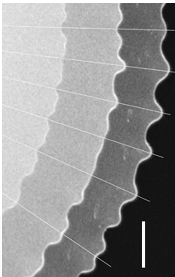
FIG. 19. Some more examples of the merging of fingers during the expansion. Drop release height is here  $H=28.8$  cm with the three flashes at 2.0, 2.6, and 3.2 ms after initial contact. The scale bar is 1 mm long. Lines have been drawn from the center of the drop to guide the eye.
