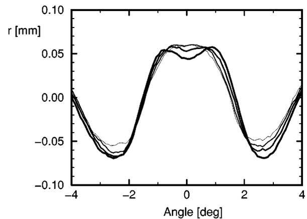
FIG. 17. The “median” shape of the fingers for four radial locations. The thickness of the lines shows the progression in time, with  $\Delta t = 0.2$  ms. The earliest shape corresponds to  $t_1 = 1.2$  ms.
