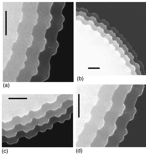
FIG. 16. Some typical examples of the splitting of fingers during the expansion. Flash spacing is  $\Delta t = 0.2$  ms in all panels. The first flash in panels (a) and (d) are 1.2 ms after contact and in (b) and (c) 1.8 ms after initial contact. The scale bars are 1 mm long.
