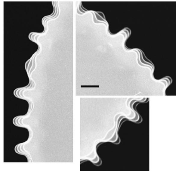
FIG. 22. The changes in the frontal undulations at maximum extent. Here  $\Delta t = 0.3$  ms, with the first flash at 5.7 ms after contact. The panels are all to the same scale and the bar is 1 mm long.
