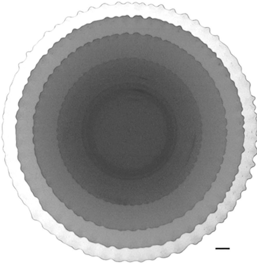
FIG. 1. A photograph (negative) showing the typical evolution of the frontal undulations during the spreading of the lamella. The four separate flashes illuminated the drop with time separation  $\Delta\tau_i=0.6$  ms, with the first flash at 1.4 ms after the initial contact. Drop diameter  $D=5.2$  mm and release height  $H=28.8$  cm. The scale bar is 1 mm long.
