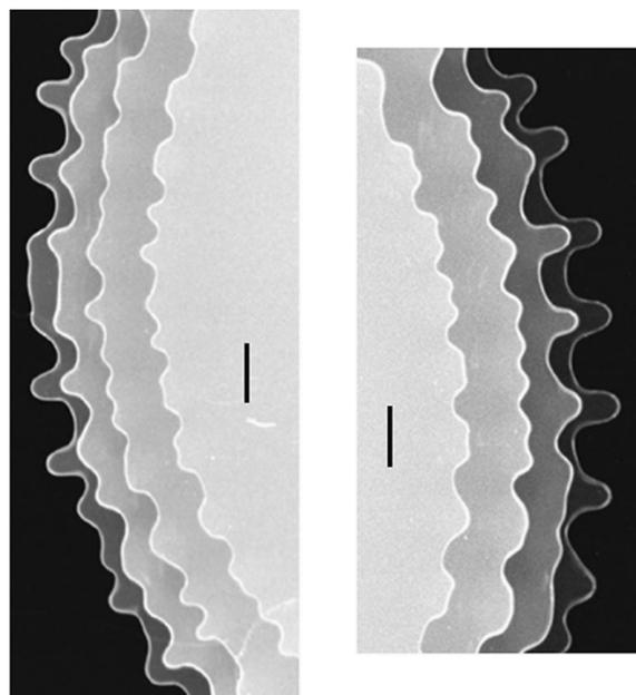
FIG. 20. The rapid evolution the frontal shapes as the drop edge nears maximum extent. The time separation of the flashes was 1.0 ms, with the first flash at 3.2 ms after contact. The two panels show two sides of the same drop. The scale bars are 1 mm long.
