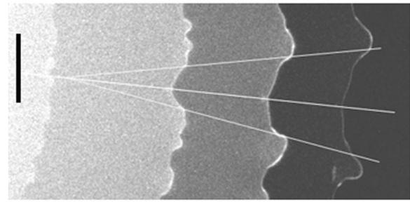
FIG. 24. Examples of large-amplitude “shock”-type disturbances at the expanding contact line. (a) Flash times are 1.2, 1.4, 1.6, and 1.8 ms after initial contact. (b) Flash times 0.2, 0.7, 1.2, and 1.7 ms after initial contact. The scale bars are 1 mm long.
