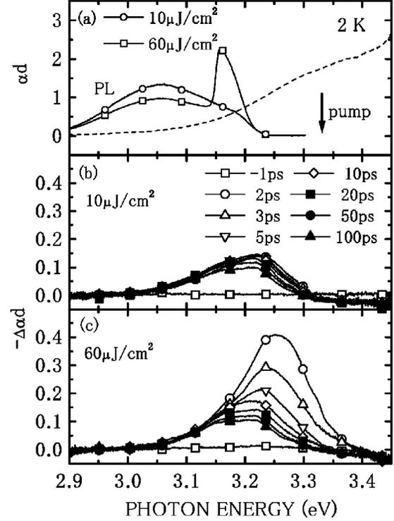
FIG. 4. The pump-and-probe measurement at 2 K. (a) The dashed line shows the absorption spectrum without pumping. The solid lines show the PL spectra under excitation densities of 10 (open circles) and  $60 \mu\text{J}/\text{cm}^2$  (open squares), respectively. The excitation photon energy is 3.323 eV. The time-resolved differential absorption spectra under excitation energy densities of (b) 10 and (c)  $60 \mu\text{J}/\text{cm}^2$ , respectively.
