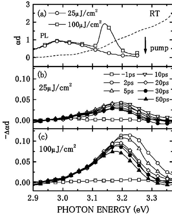
FIG. 5. The pump-and-probe measurement at RT. (a) The dashed line shows the absorption spectrum. The solid lines show the PL spectra under excitation densities of 25 (open circles) and 100  $\mu\text{J}/\text{cm}^2$  (open squares), respectively. The excitation photon energy is 3.278 eV. The time-resolved differential absorption spectra under excitation energy densities of (b) 25 and (c) 100  $\mu\text{J}/\text{cm}^2$ , respectively.
