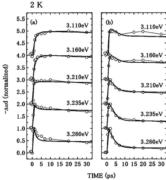
FIG. 7. Temporal changes of the differential absorption obtained under excitation energy densities of (a) 10 and (b) 60  $\mu\text{J}/\text{cm}^2$  at 2 K. Bold solid lines are calculated by the three-energy level scheme.
