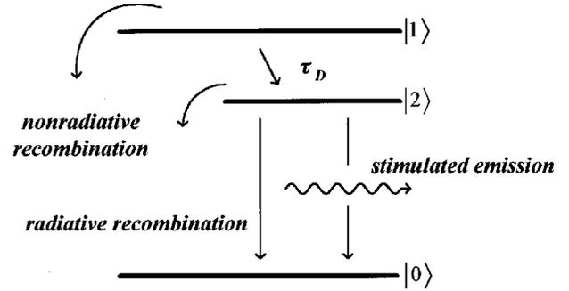
FIG. 6. Schematic illustration of the relaxation model.
