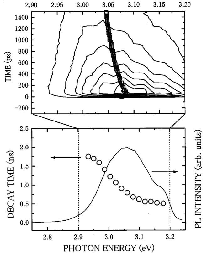
FIG. 3. (a) A contour map of the energy- and time-resolved PL intensity at 2 K. The excitation photon energy is 3.323 eV. Open squares show the PL center of the gravity as a function of time. (b) Time-integrated PL spectrum. Open circles show the decay time observed at various photon energies.
