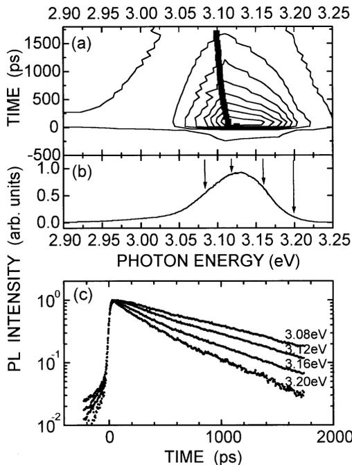
FIG. 2. (a) A contour map of the energy- and time-resolved PL intensity of sample 1 ( $x=0.08$ ). Closed squares show the PL center of gravity as a function of time. (b) Time-integrated PL spectrum. (c) Temporal change of the PL observed at 3.08, 3.12, 3.16, and 3.20 eV [indicated by arrows in (b)].
