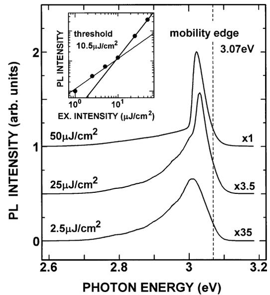
FIG. 4. PL spectra of sample 2 for different excitation energy densities. The Fabry-Perot modes are eliminated by calculation. The inset shows the excitation intensity dependence of the PL intensity. The stimulated emission appears at  $I_{\text{th}}=10.5 \mu\text{J}/\text{cm}^2$ .
