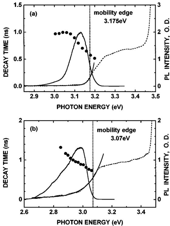
FIG. 3. (a) Absorption (a dashed line) and PL (a solid line) spectra of sample 1 ( $x=0.08$ ). They are gotten rid of by the Fabry-Perot modes and are restored by calculation. Closed circles show the decay time observed at various photon energies. The absorption tail is fitted by Eq. (1) in the text. (b) Same as (a) for sample 2 ( $x=0.14$ ).
