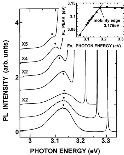
FIG. 1. PL spectra of sample 1 ( $x=0.08$ ) under the site-selective excitation (3.122~3.305 eV). Closed circles show the PL peaks. The inset shows the PL peak energy as a function of the excitation photon energy.
