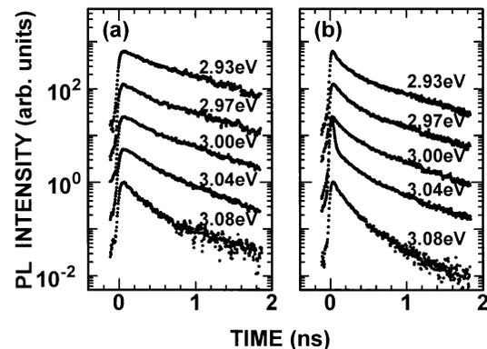
FIG. 5. (a) Time-resolved PL under the low-density excitation  $I_{\text{ex}}=2.5 \mu\text{J}/\text{cm}^2$ . (b) Time-resolved PL under the high-density excitation  $I_{\text{ex}}=25 \mu\text{J}/\text{cm}^2$ .
