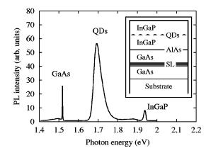
FIG. 1. PL spectrum of the sample QDP1779. "QDs," "InGaP," and "GaAs" mark PL of the QDs and of the excitons of the barrier and buffer layers, respectively. Inset: structure of the studied samples.
