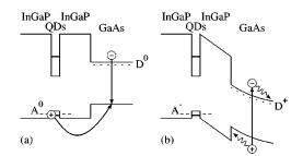
FIG. 3. Charge transfer during the structure growth (a) and the optical pumping (b).
