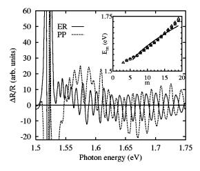
FIG. 2. Pump-probe (PP) and electroreflection (ER) spectra of the sample QDP1779. Inset: the energy position of FKO maxima vs their numbers for the samples QDO1504 ( $\bigcirc$ ), QDO1505 ( $\times$ ), and QDP1779 ( $\triangle$ ). Solid line is fitting by formula (1) with a parameter F = 30 kV/cm.
