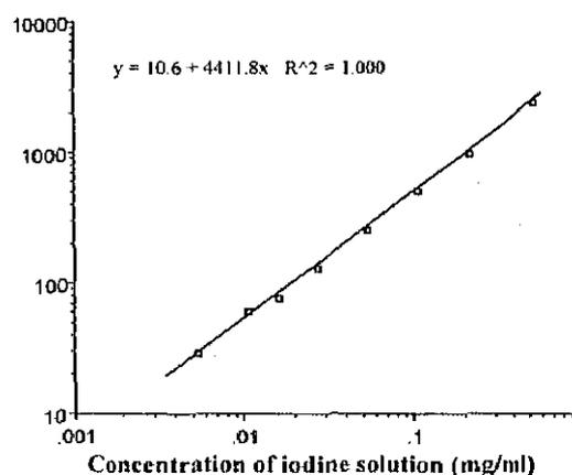
**Fig.2 The relationship between fluorescent x-ray counts and iodine concentration**
