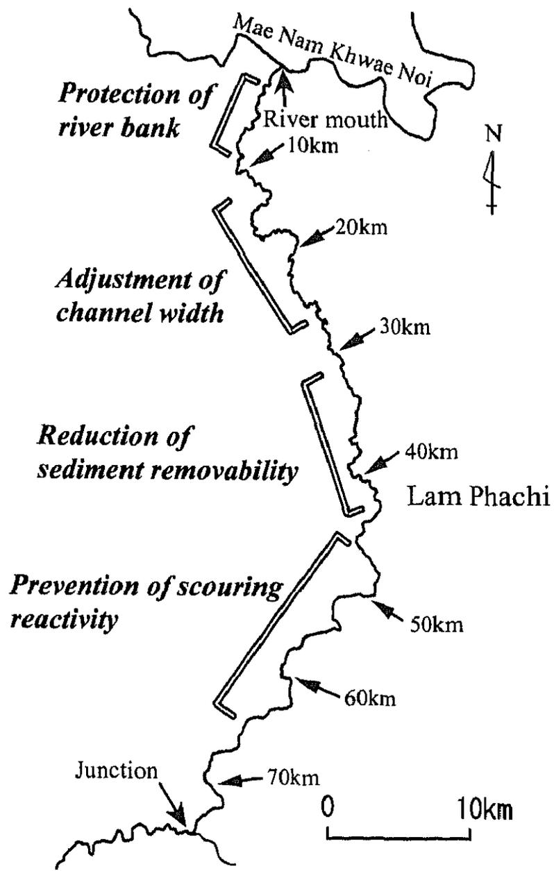
Fig. 8 Proposals to prevent sediment disasters and flooding
