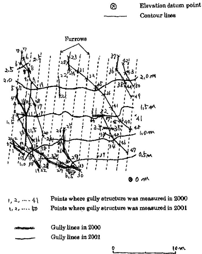
Fig. 1 Gully lines in a pineapple field
