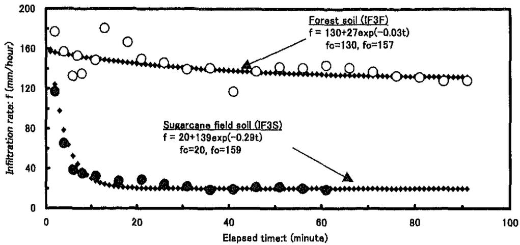
Fig. 12 Infiltration capacity curves of the forestland and the sugarcane field at the IF3 site
