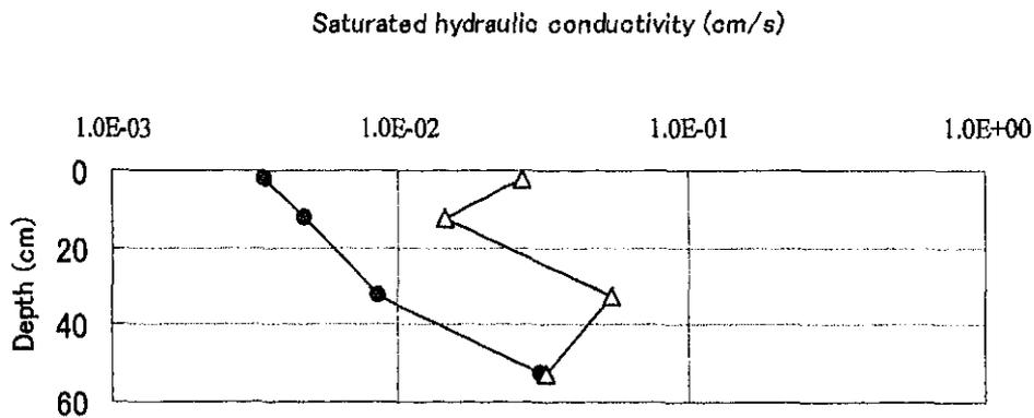
Fig. 4 Saturated hydraulic conductivity at each depth
