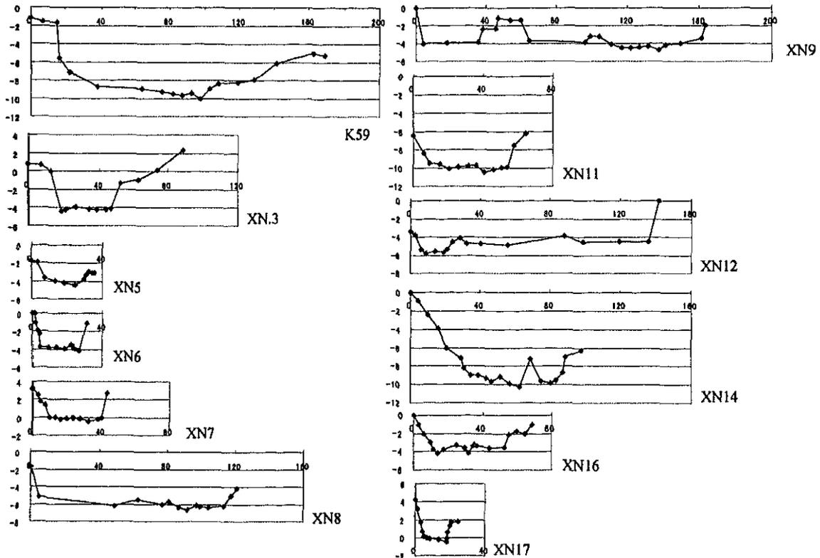
**Figure 4. Cross section along Lam Phachi main channel**
