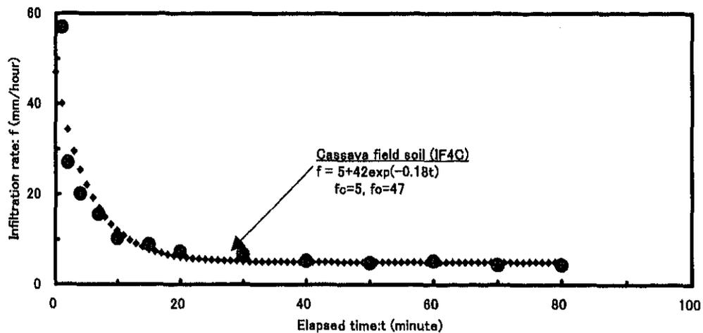
Fig. 13 Infiltration capacity curve of the cassava field at the IF4 site
