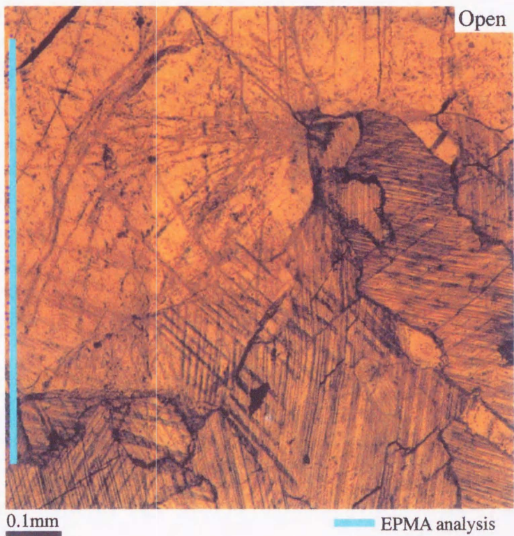
Fig. 8. Cathodoluminescence image (upper) and microphotograph under open nicol (lower) of group-C limestone ( \delta^{18}\text{O}=7.1\text{‰} and \delta^{13}\text{C}=-0.8\text{‰} ) collected from the drill core of 7MAKK-1. EPMA analysis for the determination of MnO content in calcite was made along a blue line in the lower photograph.
