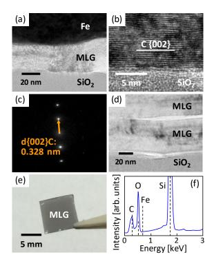
**Fig. 2.** Characteristics of the normal layer exchange sample formed at 1000 °C. (a) Cross-sectional bright-field TEM image. (b) High-resolution lattice image of the MLG layers showing a substrate-contacted region. (c) SAED pattern with a selected area of 200 nm diameter. (d) Bright-field TEM image showing an island area. (e) Photograph and (f) EDX spectrum of the sample after Fe removal.
