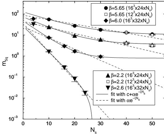
Figure 1.  $m_{5q}$  as a function of  $N_s$  at  $a^{-1} \simeq 1$  GeV and  $m_0 = 1.7$  and at  $a^{-1} \simeq 2$  GeV and  $m_0 = 1.8$ , where  $m_0$  is the domain-wall height, for the plaquette ( $\beta = 5.65, 6.0$ ) and RG-improved ( $\beta = 2.2, 2.6$ ) gauge action [5].
