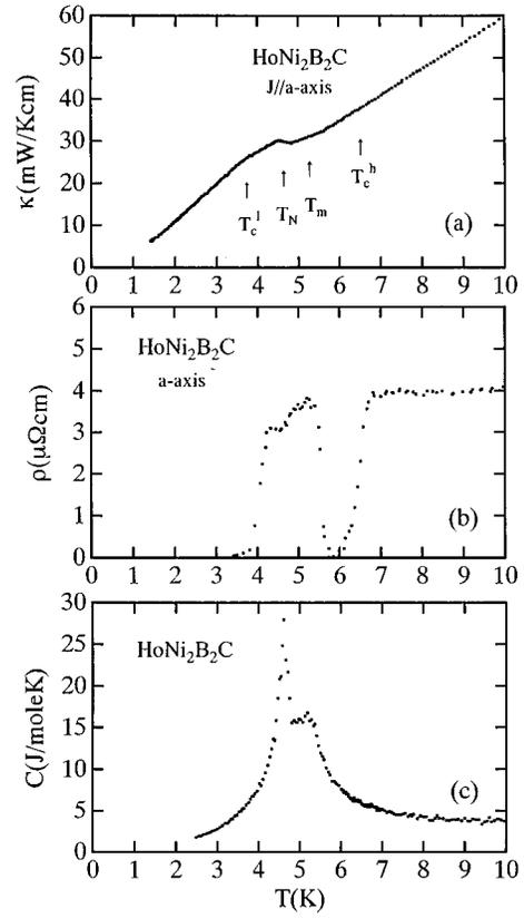
FIG. 4. Temperature dependence of (a) the thermal conductivity, (b) electrical resistivity, and (c) specific heat of  $\text{HoNi}_2\text{B}_2\text{C}$  at low temperatures.  $T_c^h$  and  $T_c^l$  are the higher and lower superconducting transition temperatures, respectively, and  $T_m$  and  $T_N$  are the incommensurate and commensurate antiferromagnetic transition temperatures, respectively.
