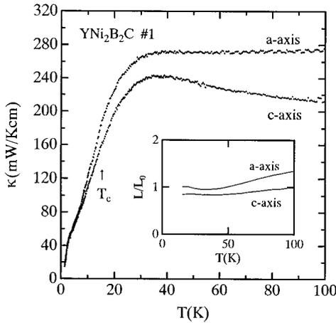
FIG. 1. Temperature dependence of the thermal conductivity with heat current  $J$  parallel to the  $a$  and  $c$  axes of  $\text{YNi}_2\text{B}_2\text{C}$ , sample 1. The inset shows the temperature dependence of the reduced Lorenz number  $L/L_0$  of sample 1. See the text in detail.
