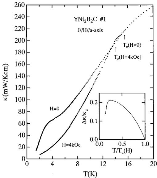
FIG. 2. Temperature dependence of the thermal conductivity with heat current  $J$  parallel to the  $a$  and  $c$  axes of  $\text{YNi}_2\text{B}_2\text{C}$  sample 1 under the longitudinal magnetic field. The inset shows the temperature dependence of the difference of the temperature dependence of the thermal conductivities  $\kappa_c$  normalized at  $T_c(H)$  between under  $H=0$  and  $H=4$  kOe.
