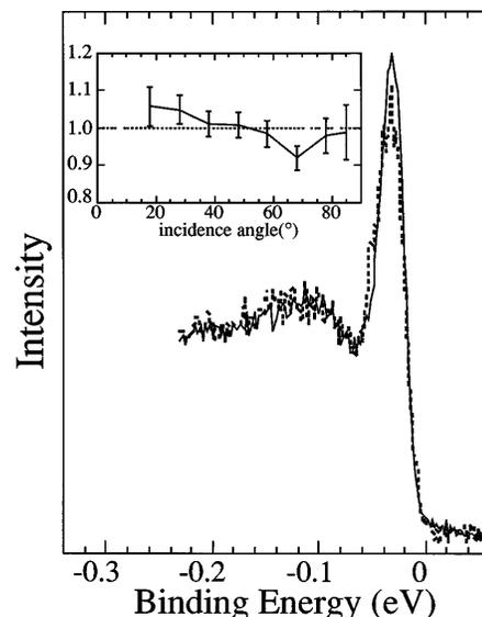
FIG. 3. Low temperature ( $T = 13$  K) EDC's of Bi2212 at  $\bar{M}$  for various incident photon angles. The solid (dashed) line is  $18^\circ$  ( $85^\circ$ ) from the normal. The inset shows the height of the sharp peak for data normalized to the broad peak at different incident angles.
