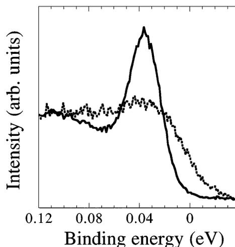
FIG. 1. Comparison of data at  $\bar{M}$  in the normal state (105 K, dashed line) and the superconducting state (13 K, solid line) for a slightly overdoped ( $T_c = 87$  K) Bi2212 sample with photon polarization  $\Gamma - \bar{M}$ .
