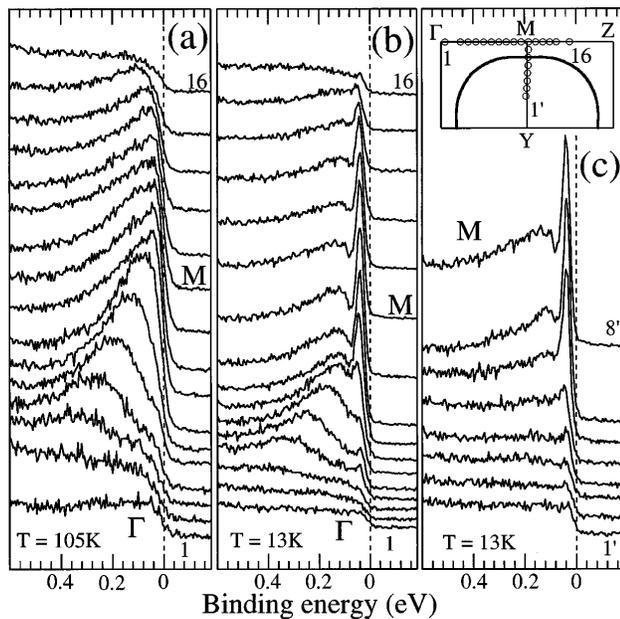
FIG. 2. EDCs in (a) the normal state (105 K) and (b) the superconducting state (13 K) along the line  $\Gamma - \bar{M} - Z$ , and (c) the superconducting state (13 K) along the line  $\bar{M} - Y$ , with the same sample and photon polarization as in Fig. 1. The zone is shown as an inset in (c) with the curved line representing the observed Fermi surface.
