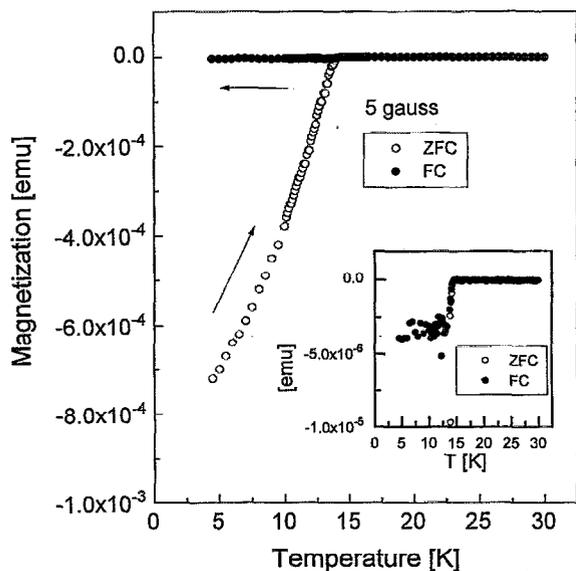
FIG. 3. Temperature dependence of the magnetization of the  $\text{Y-Ni-B-C}$  thin film measured in a magnetic field of 5 G perpendicular to the film plane. The arrows represent warming process after cooling in zero field, and cooling process in the field. Inset shows the expanded view of the field cool data.
