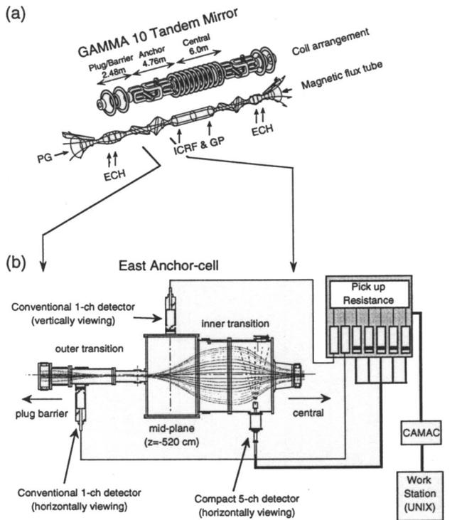
FIG. 1. The schematic view of GAMMA 10 and the location of the  $H_{\alpha}$  diagnostic system. (a) The GAMMA 10 coil system and the shape of the magnetic flux tube, together with the location of the plasma production and heating systems.
