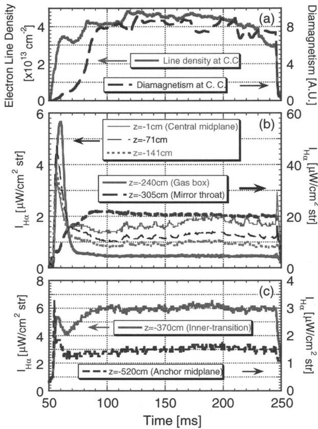
FIG. 3. Temporal behavior of the intensity in the  $H_{\alpha}$  emission measured in the region from the central-cell to the east anchor-cell, together with the line-density and diamagnetism at the central-cell. (a) Electron line-density and diamagnetism at the central-cell. (b)  $H_{\alpha}$  intensity measured at various positions in the central-cell. (c)  $H_{\alpha}$  intensity in the anchor-cell.
