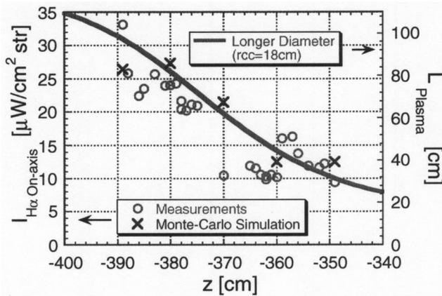
FIG. 5. Axial profile of  $H_{\alpha}$  intensity measured in the east inner-transition region and comparison with the simulation result. Circle is the measured result, cross represents the simulation results, and the solid curve shows the length of the longer axis of the plasma cross section.
