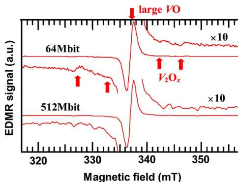
FIG. 2. (Color online) Typical EDMR spectra measured for JLCs of 64 and 512 Mbit samples (80 nA at  $V_R=9.6$  V and 55 nA at  $V_R=5.9$  V, respectively) at room temperature with the magnetic field parallel to [011] axis.
