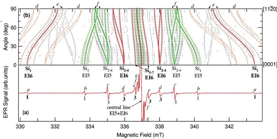
FIG. 1. (Color online) EPR measurements of electron-irradiated *p*-type 4H-SiC at 150 K. (a) EPR spectrum for  $\mathbf{B}||[0001]$ . (b) Angular dependence of signal positions for  $\mathbf{B}$  rotation in the  $(\bar{1}100)$  plane. Solid lines were calculated using the spin-Hamiltonian parameters given in Table I.
