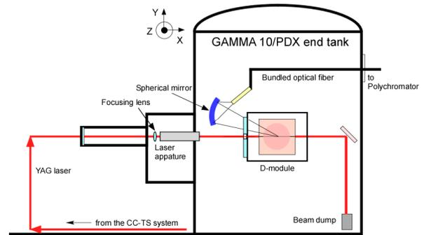
Fig. 3 Schematic view of the end-TS system.
