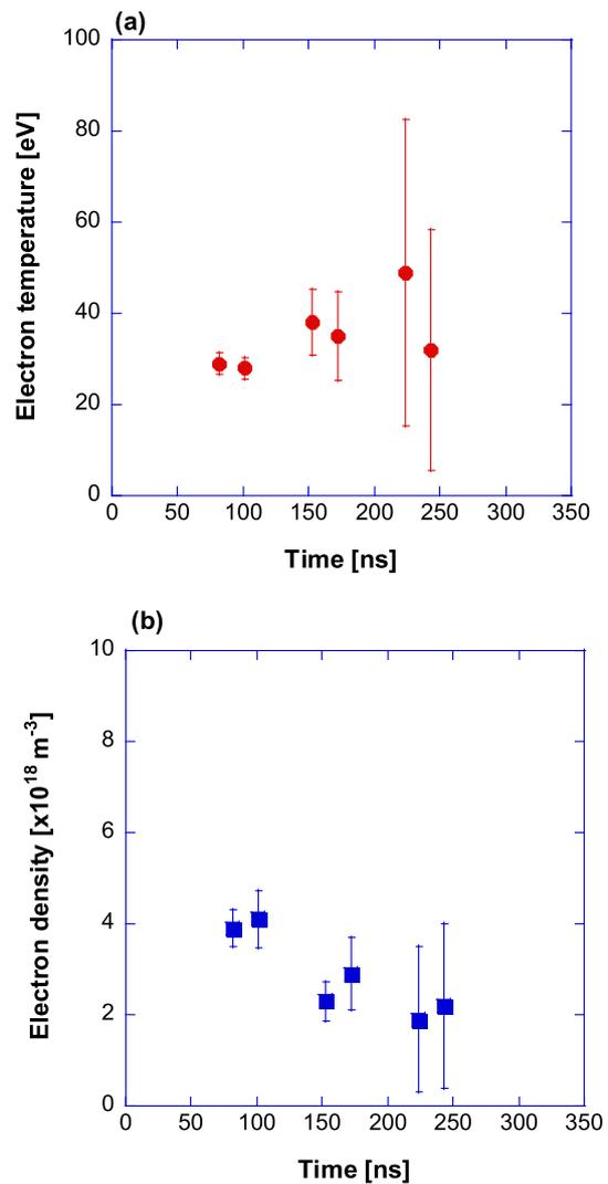
Fig. 9 Time-dependent (a) electron temperature and (b) density measured by the multi-pass TS system at  $t = 151.5$  ms.
