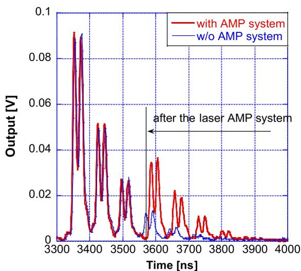
Fig. 5 Rayleigh scattering signals of the multi-pass system.
