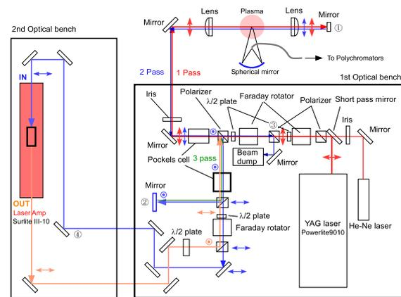
Fig. 4 Schematic diagram of the multi-pass TS system with the amplification system.
