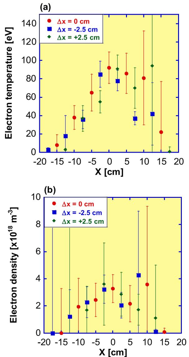
Fig. 6 Radial (a) electron temperature and (b) density.
