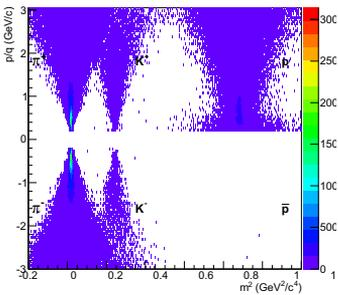
Fig. 3. Rigidity ( $p/q$ ) (GeV/c) vs mass-squared ( $\text{GeV}^2/c^4$ ).
