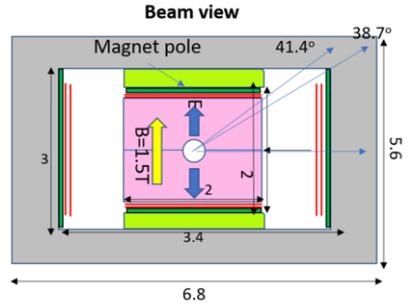
Fig. 2. The beam view of the hadron spectrometer.
