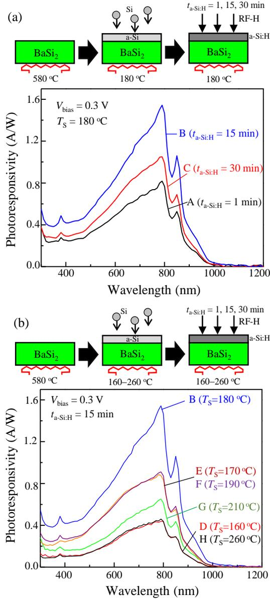
FIG. 2 (a) Photoresponsivity spectra of 500 nm-thick  $\text{BaSi}_2$  layers capped with approximately 3 nm-thick  $\text{a-Si:H}$  fabricated with various  $t_{\text{a-Si:H}}$ . (b) Photoresponsivity spectra of 500 nm-thick  $\text{BaSi}_2$  layers capped with approximately 3 nm-thick  $\text{a-Si:H}$  fabricated with various  $T_S$ .
