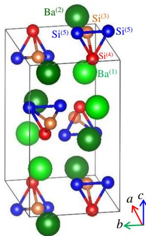
FIG. 1. Crystal structure of orthorhombic BaSi<sub>2</sub>. There are three inequivalent Si sites and two inequivalent Ba sites.
