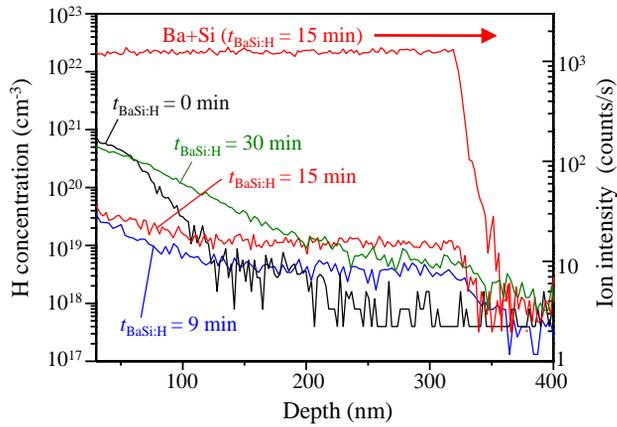
FIG. 4. SIMS depth profiles of H atoms of approximately 300 nm-thick  $\text{BaSi}_2$  films with various values of  $t_{\text{BaSi:H}}$  in the range of 0–30 min at  $T_S = 580$  °C. Depth profiles of ions (Ba and Si) of  $\text{BaSi}_2$  films with  $t_{\text{BaSi:H}} = 15$  min is also shown.
