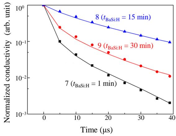
FIG. 6. Normalized photoconductivity of  $\text{BaSi}_2$  versus time. Comparison of experimental data (samples 7-9) with theoretical estimations obtained by the approach using Eqs. (1), (4), (5) and (6). Photoconductivity is normalized to the value at  $t = 0$ .
