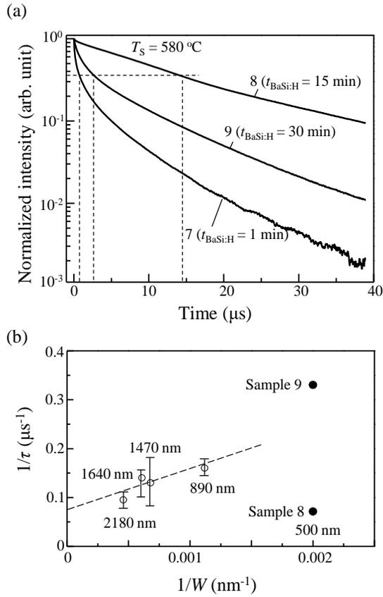
FIG. 5. (a) Photoconductivity decay curves of atomic H-passivated BaSi<sub>2</sub> films in samples 7-9, fabricated using different  $t_{\text{BaSi:H}}$ . (b) Comparison of  $\tau$  obtained for samples 8 and 9 as a function of BaSi<sub>2</sub> thickness  $W$  to those reported previously [8].
