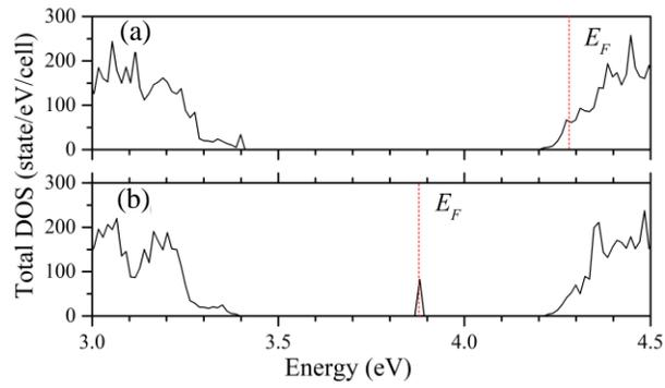
FIG. 8. Total density of states of an enlarged  $\text{BaSi}_2$  unit cell with one H in different interstitial positions indicating (a) degenerate semiconducting properties and (b) the appearance of a trap in the gap region.
