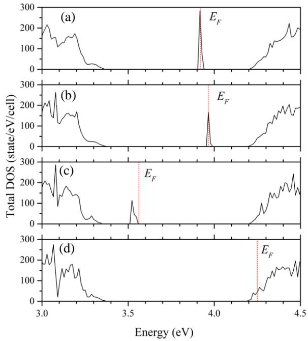
FIG. 7. Total density of states of enlarged  $\text{BaSi}_2$  unit cells with (a) one Si vacancy, (b) one H atom in a Si vacancy, (c) two H atoms in a Si vacancy, and (d) three H atoms in a Si vacancy. The vertical dashed line indicates the Fermi level.
