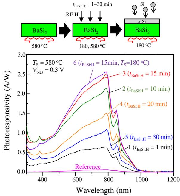
FIG. 3. Photoresponsivity spectra of 500 nm-thick  $\text{BaSi}_2$  layers passivated by atomic H with various values of  $t_{\text{BaSi:H}}$  in the range of 0–30 min.
