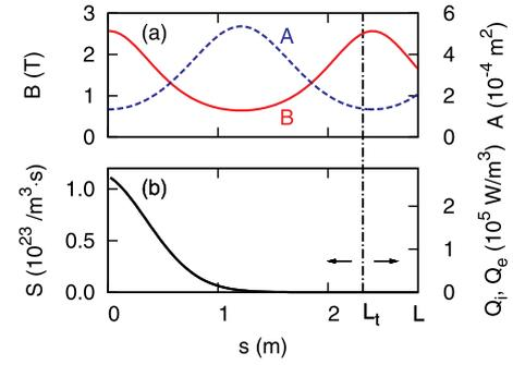
Fig. 1. Calculation conditions used in this study; parallel-to-B profiles of (a) the magnetic field strength  $B$  (solid line), the cross-sectional area of the flux tube  $A$  (broken line) and (b) source terms. The vertical chain line represents the target position.
