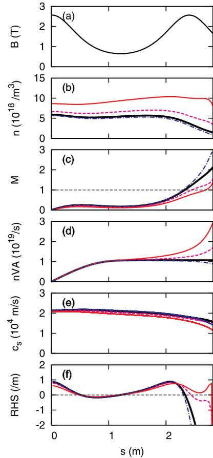
**Fig. 6.** Profiles of (a)  $B$ , (b)  $n$ , (c)  $M$ , (d) the area-integrated particle flux  $nVA$ , (e)  $c_s$  and (f) the right hand side of Eq. (4) for  $S_{\text{add}} = 0$  (thick solid lines,  $R = 1$ ),  $3S_0$  (thin solid lines,  $R \sim 2.75$ ),  $S_0$  (thin broken lines,  $R \sim 1.58$ ),  $-0.3S_0$  (thin chain lines,  $R \sim 0.83$ ).
