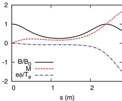
**Fig. 3.** Profiles of normalized magnetic field strength  $B/B_0$  (solid line), Mach number  $M$  (broken line) and normalized electrostatic potential  $e\phi/T_e$  (chain line) obtained from the AIP model.
