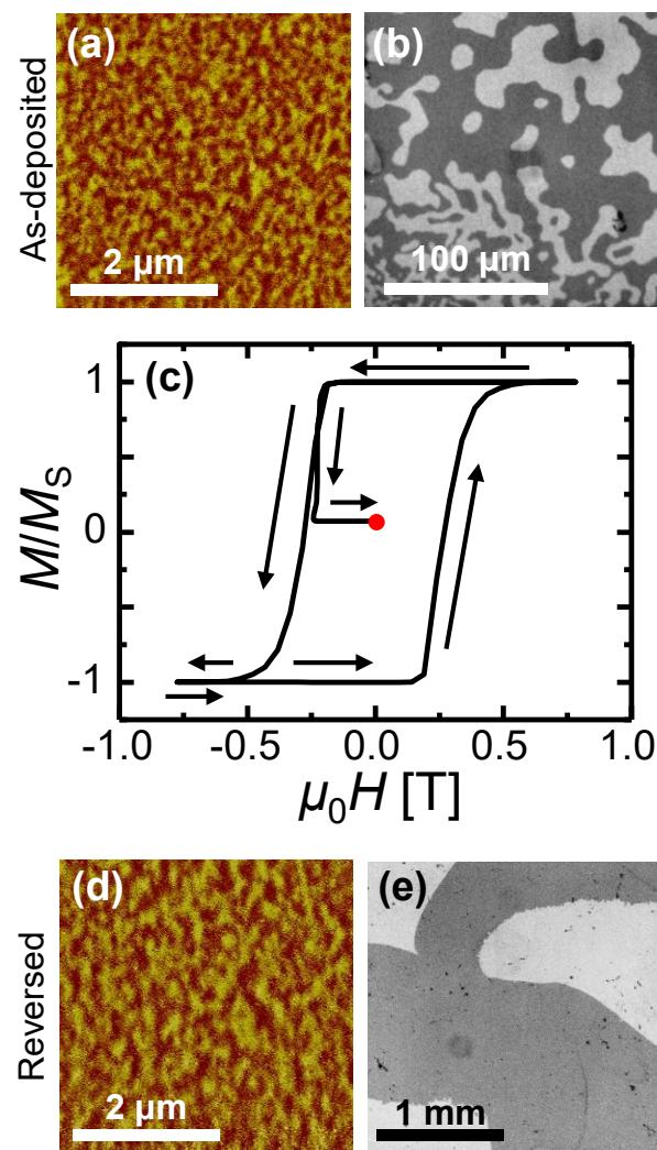
Fig. 3 (a) MFM image of the Mn<sub>4</sub>N/MgO and (b) MOKE image of the Mn<sub>4</sub>N/STO samples in the as-deposited state. (c) Magnetization curve illustrating the partial reversal process, monitored by extraordinary Hall effect in the Mn<sub>4</sub>N/STO sample. The red dot corresponds to the final magnetization state, used for (e). (d) MFM image of the Mn<sub>4</sub>N/MgO sample and (e) MOKE image of the Mn<sub>4</sub>N/STO sample after partial reversal.
