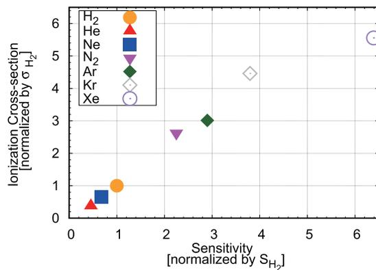
Fig. 4 Electron-impact ionization cross sections of gases normalized against hydrogen plotted against the relative sensitivities of the AIG.
