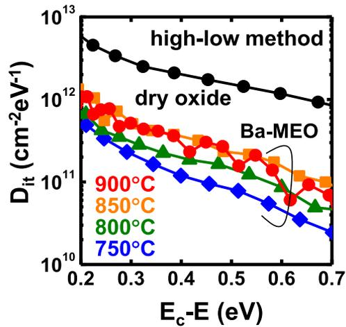
FIG. 3. Change in the energy distribution of  $D_{it}$  for Ba-incorporated SiC-MOS capacitors depending on the MEO temperature. Ba-MEO was conducted at various temperatures ranging from 750 to 900°C for 4 h.  $D_{it}$  values were estimated using a high-low method. All SiO<sub>2</sub>/SiC structures received POA prior to electrode deposition.  $D_{it}$  distribution taken from the reference device with a thermal oxide (dry oxide) grown at 1150°C [20] was also shown.
