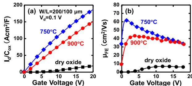
FIG. 4. Basic performance of Ba-incorporated SiC-MOSFETs fabricated with MEO at 750 or 900°C for 1 h: (a)  $I_d$ - $V_g$  characteristics normalized by  $C_{ox}$ , and (b)  $\mu_{FE}$  extracted from the transfer characteristics. Results from a reference thermal oxide (dry oxide) formed at 1300°C without Ba incorporation are also shown. The gate width and length of the devices (W/L) and drain voltage for  $I_d$ - $V_g$  measurements are indicated.
