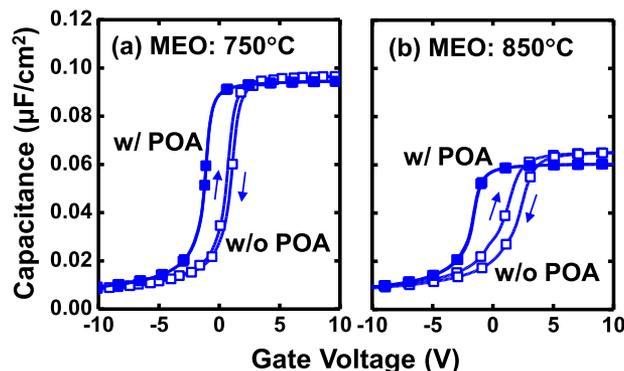
FIG. 2. Typical bidirectional C-V characteristics of Ba-incorporated SiC-MOS capacitors fabricated by MEO with a 0.1-nm-thick Ba interfacial layer at (a)  $750^\circ C$  and (b)  $850^\circ C$  for 4 h. Results with and without POA in  $N_2$  ambience are indicated by the filled and open symbols, respectively.
