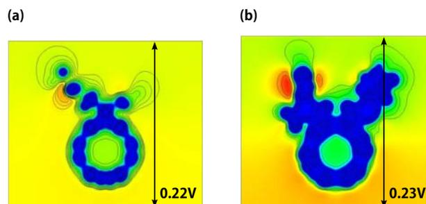
Figure 2: Contour plots of the electrostatic potential of neutral (a) PCBM and (b) SIMEF. Each contour represents higher or lower by 0.01 in the density of the adjacent contour lines.
