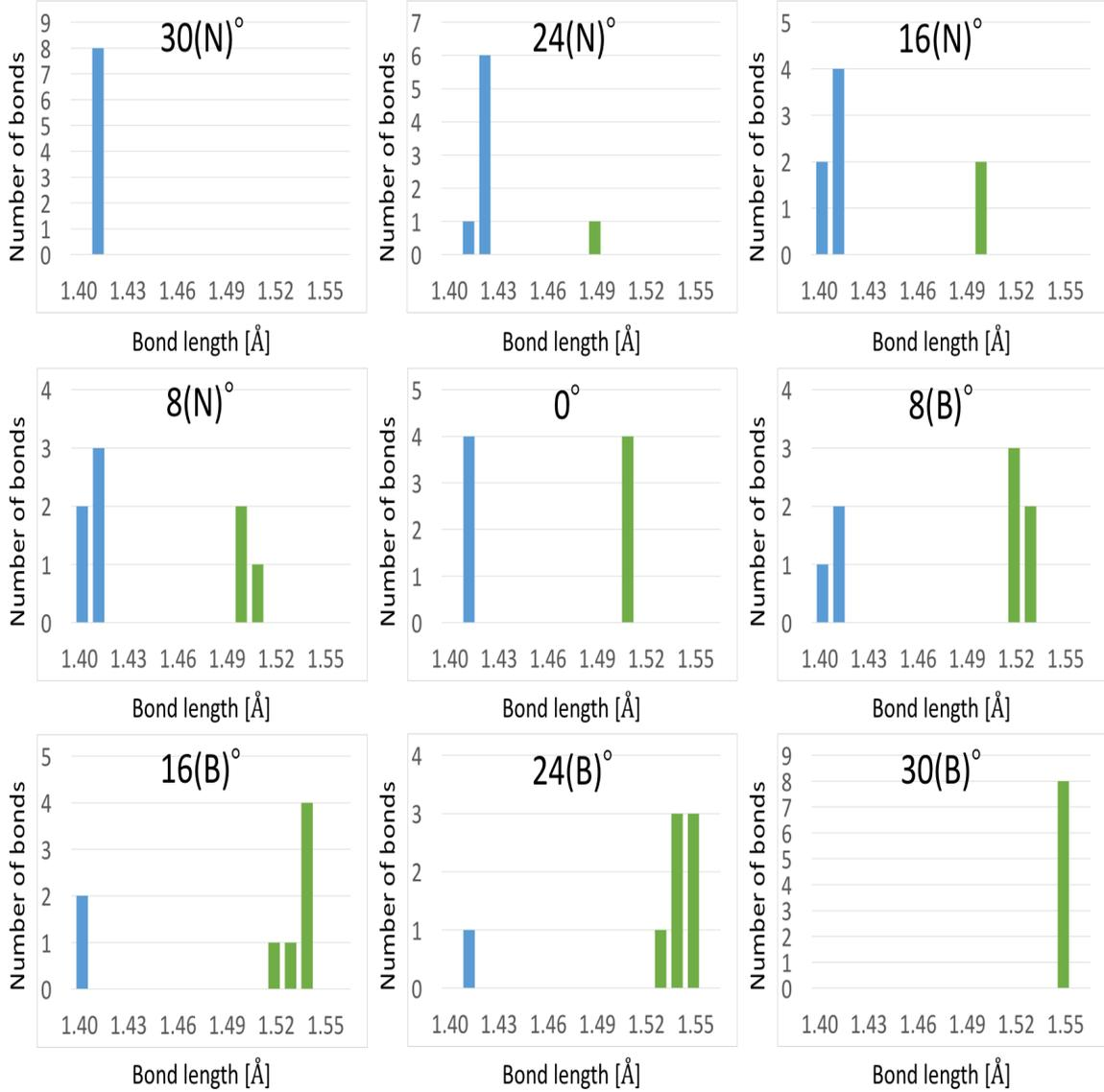
**Fig. 3.** Distribution of the bond length at the border of the heterostructures consisting of h-BN and graphene strips. Green and blue bars indicate the distribution of the bond length of BC and NC heterobonds, respectively. Border angles of  $\theta(N)$  and  $\theta(B)^\circ$  indicate the border angle  $\theta$  consisting mainly of NC and BC heterobonds, respectively. The  $\theta = 0^\circ$  corresponds with the armchair border.
