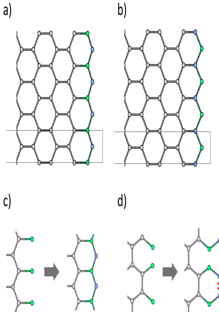
**Fig. 4.** Optimized structures of graphene with zigzag edges adsorbing a BN with (a) BC and (b) NC heterobonds. Black lines indicate the unit cell of the structures. Schematic views of formation of the first and second formation steps of h-BN at (c) the zigzag and (d) armchair edges of graphene. Green, gray, and blue circles indicate B, C, and N atoms, respectively.
