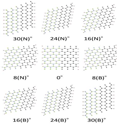
**Fig. 1.** Optimized geometries of nanoribbons consisting of h-BN and graphene nanostrips with the BC zigzag ( $30(\text{B})^\circ$ ), BC dominant chiral ( $24(\text{B})$ ,  $16(\text{B})$ , and  $8(\text{B})^\circ$ ), nonpolar armchair ( $0^\circ$ ), NC dominant chiral ( $24(\text{N})$ ,  $16(\text{N})$ , and  $8(\text{N})^\circ$ ), and NC zigzag ( $30(\text{N})^\circ$ ) borders. Green, black, blue, and pink circles denote B, C, N, and H, respectively.
