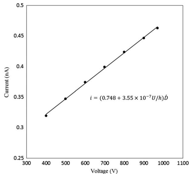
Fig. 3. Electric current as a function of applied voltage. The line represents the linear fitting result of the measured values. The dose per pulse  $\dot{D}$  was 0.296 mGy at the depth of the sensitive volume.
