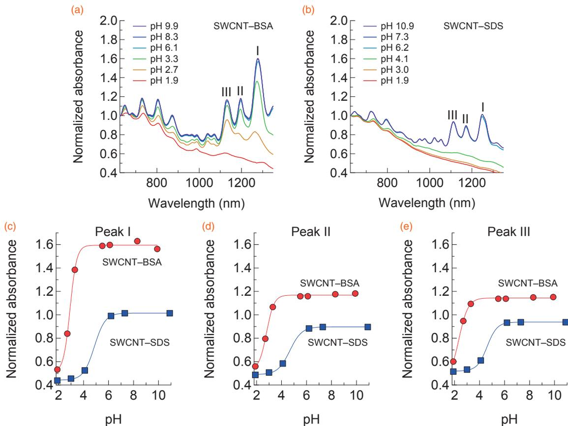
**Fig. 2.** pH dependence of the absorbance spectra of SWCNT-BSA (a) and SWCNT-SDS (b), which were normalized to the absorbance at 625 nm. Normalized absorbances of SWCNT-BSA and SWCNT-SDS at peaks I (c), II (d), and III (e) as a function of pH.
