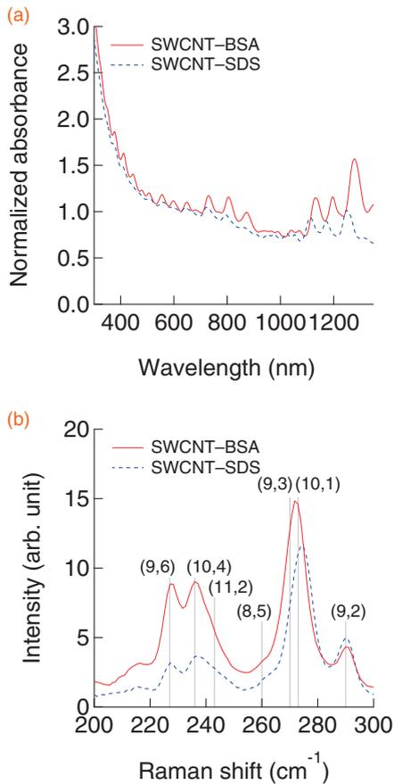
**Fig. 1.** (a) Absorption spectra of SWCNT-BSA and SWCNT-SDS samples normalized to the absorbance at 625 nm. (b) Raman spectra of SWCNT-BSA and SWCNT-SDS samples with an excitation wavelength of 532 nm. The peak positions were determined by decomposition using fitting by the Lorentzian function.
