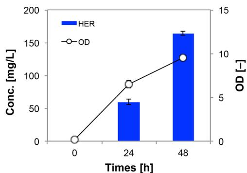
**Figure 5.** Culture profiles of strain ET1. *E. coli* BW25113 harboring pCF1s-MsD (strain ET1) was cultured in M9Y medium supplemented with L-His and L-Met. After 3 h of cultivation, 0.5 mM IPTG was added to the medium. Data are presented as mean values with standard errors from three independent experiments.
