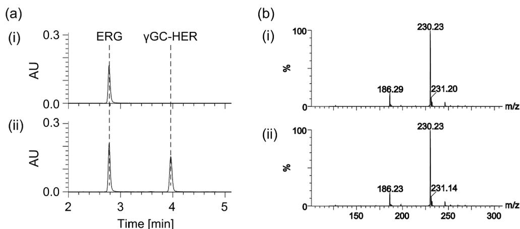
**Figure 4.** LC-ESI-MS analysis of EgtE reaction products. (a) Traces at 250 nm of (i) ERG standard and (ii) reaction products. The reaction (40  $\mu$ L) was carried out by adding purified recombinant EgtE (2.5  $\mu$ M) and EgtC (3.9  $\mu$ M) (ii) to the boiled supernatant of the EgtB reaction mixture containing 2 mM dithiothreitol at 25  $^{\circ}$ C for 17 h. (b) MS spectra of (i) ERG standard and (ii) EgtE reaction product (ESI positive mode).
