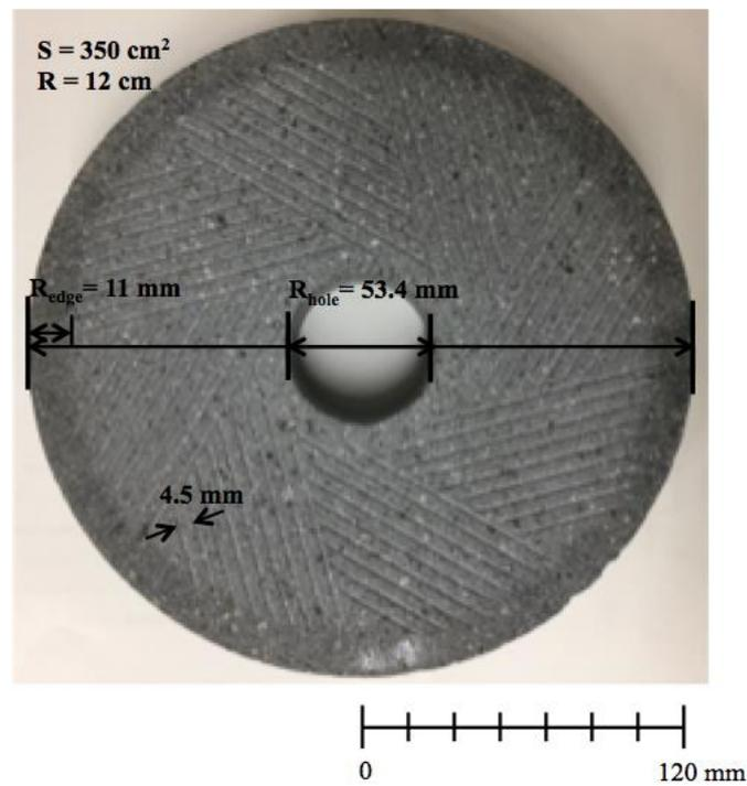
**Fig. 2.** The lower millstone of the Mill with contact surface area of  $350 \text{ cm}^2$ , millstone radius of 12 cm, edge distance of 11 mm, and groove width of 4.5 mm. The upper millstone is the same as the lower millstone.
