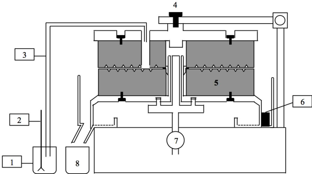
**Fig. 1.** Micro wet milling (MWM) system. (1) Raw material; (2) Stirrer; (3) Tubing pump; (4) Gap controller; (5) Lower millstone; (6) Rubber spatula; (7) Electric motor; (8) Sample receiver.
