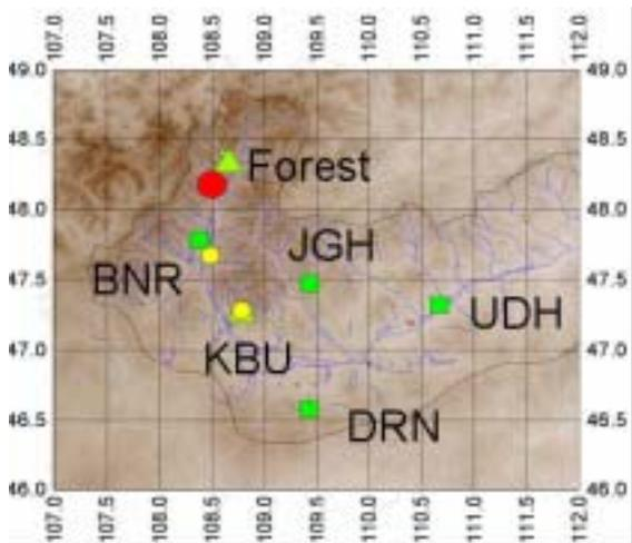
**Fig. 1** Observation stations in upper Kherlen River basin. Triangles denote flux stations, rectangular AWSs, small circles hillslope observation sites, larger circle the GPS station.
