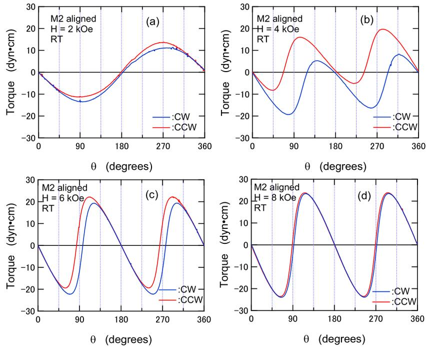
FIG. 3. Typical magnetic torque curves for the aligned  $\alpha''$ - $\text{Fe}_{16}\text{N}_2$  particles sample (M2) at an external field of (a) 2 kOe, (b) 4 kOe, (c) 6 kOe, and (d) 8 kOe. Rotational hysteresis was clearly observed in the curves below 6 kOe.
