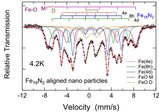
FIG. 2. Mossbauer spectrum for the  $\alpha$ - $\text{Fe}_{16}\text{N}_2$  aligned sample recorded at 4.2 K. Solid lines show the results of the fit. Corresponding peak positions are indicated by three bars for magnetic subspectra of the  $\alpha''$ - $\text{Fe}_{16}\text{N}_2$  core and two bars, magnetic sextet (M), and paramagnetic doublet (D), for the outer shell of Fe oxides (Fe-O).
