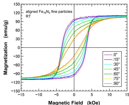
FIG. 1. Magnetization curves of the  $\alpha''$ -Fe<sub>16</sub>N<sub>2</sub> aligned sample. The external magnetic field was applied with an angle from the magnetic alignment direction. The angle ranged from 0 to 90° and coercive fields decreased monotonically with an increase of the angle. Data were partly shown in a previous report.<sup>13</sup>
