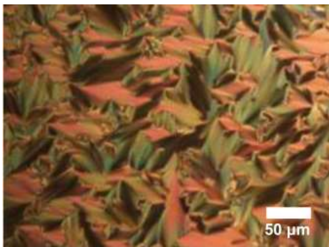
Figure 1. Polarizing optical microscopy (POM) image of blend cholesteric LC (sesamin 3 mol% in 6CB).
