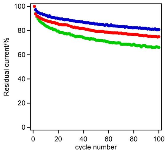
**Figure 8.** Stability of the electrode response during rotation at 10,000 rpm for the various pore morphologies (macropore/mesopore ratio) at 15 °C. MgOC<sub>meso</sub> (blue), MgOC<sub>macro</sub> (green), and MgOC<sub>33</sub> (red).
