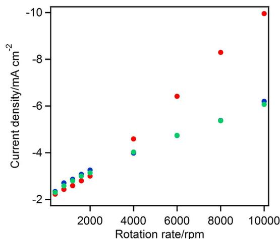
**Figure 6.** Rotation rate dependence of the current density. MgOC<sub>macro</sub> (green), MgOC<sub>33</sub> (red), and MgOC<sub>meso</sub> (blue).
