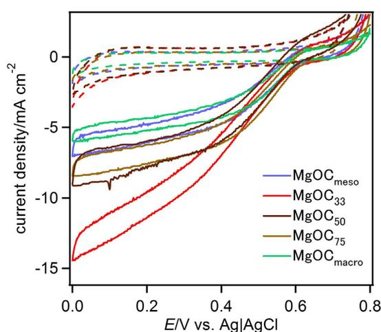
**Figure 4.** CV data for BOD adsorbed on a  $\text{MgOC}$ -modified electrode in a citrate buffer (0.1 M, pH 5.0) under  $\text{O}_2$ -saturated conditions at 25 °C (solid curve).  $\text{MgOC}_{\text{meso}}$  (blue),  $\text{MgOC}_{33}$  (red),  $\text{MgOC}_{50}$  (blue),  $\text{MgOC}_{75}$  (purple),  $\text{MgOC}_{\text{macro}}$  (green). The scan rate was  $1 \text{ mV s}^{-1}$ . Dashed curves indicate CVs without BOD.
