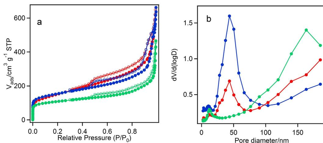
**Figure 2.** (a)  $N_2$  adsorption (closed circle) and desorption (open circle) isotherms and (b) the pore size distribution of MgOCs analysed by the BJH method.  $MgOC_{meso}$  (blue),  $MgOC_{macro}$  (green),  $MgOC_{50}$  (red).
