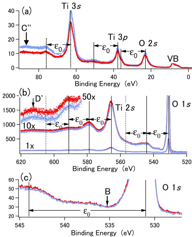
FIG. 6. (a) O 2s, Ti 3p, and Ti 3s spectra for the  $\beta$  (blue) and  $\lambda$  (red) phases. (b) O 1s and Ti 2s spectra for the  $\beta$  (gray, thin blue) and  $\lambda$  (black, red) phases. (c) O 1s spectra on an enlarged vertical scale.
