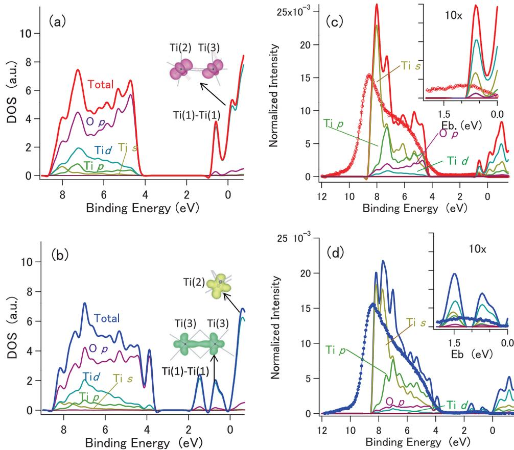
FIG. 2. (a) and (b) DOSs and PDOSs. (c) and (d) Comparisons of experimental and simulated spectra for the  $\lambda$  phase [(a) and (c)] and  $\beta$  phase [(b) and (d)], respectively. The experimental and simulated  $t_{2g}$  spectra are shown on enlarged scales in the inset to (c) and (d).
