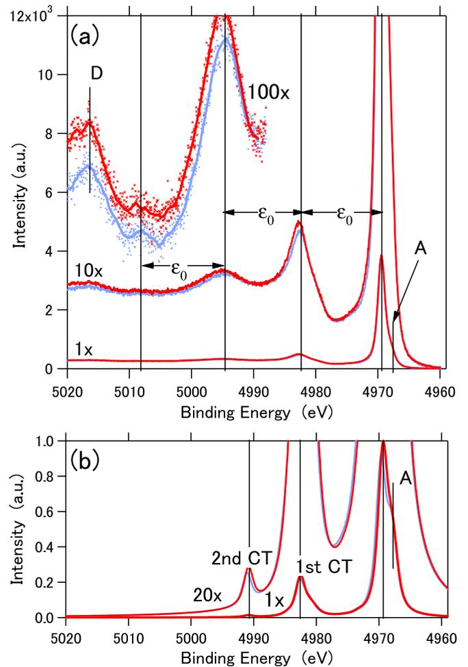
FIG. 5. Experimental (a) and simulated (b) Ti  $1s$  spectra, shown at different vertical magnifications. In the highest magnification (100 $\times$ ) experimental spectra, the data points are shown by dots, and 30 point smoothed spectra are shown by solid curves. The gray and black (thin blue and red) represent the  $\beta$  and  $\lambda$  phases, respectively.
