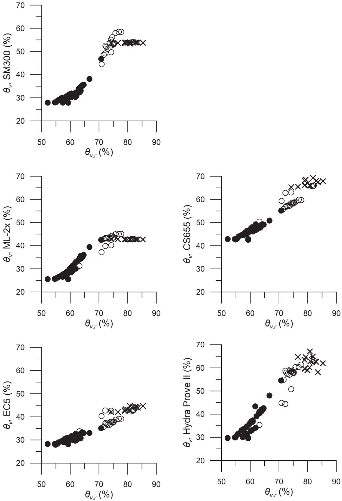
Fig. 2 Relation between the  $\theta_v$  values measured by the five sensors and the reference  $\theta_{v,r}$  values from the weight measurement. Closed circles indicate those for  $\text{bulk EC} \leq 1.5$  dS/m, open circles for  $1.5 < \text{bulk EC} \leq 2.5$  dS/m, and crosses for  $2.5 \text{ dS/m} < \text{bulk EC}$ .
