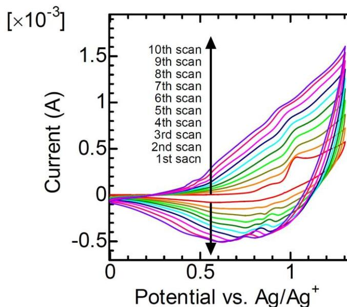
FIGURE 2 Cyclic voltammetry (CV) result in 10 scans versus Ag/Ag<sup>+</sup> reference electrode during polymerization under circularly polarized light. Polymerization under pulse L-CPL at 532 nm.
