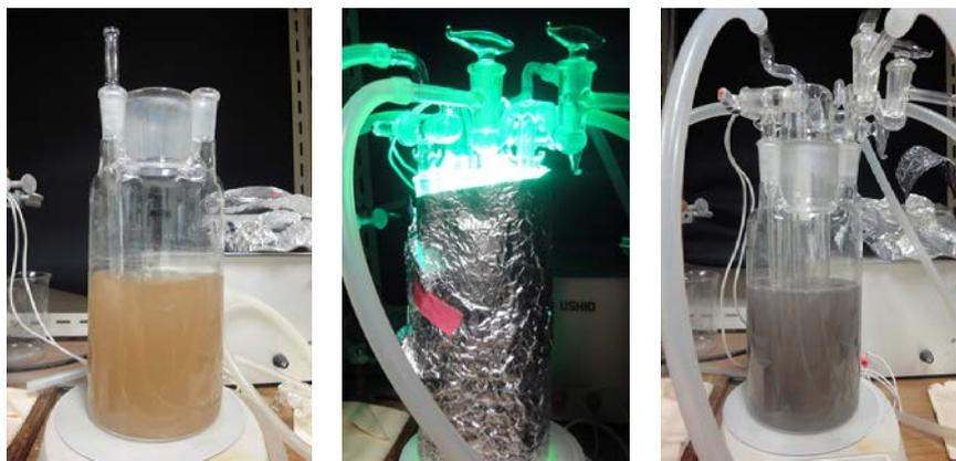
(a) Before irradiation, (b) under UV irradiation and (c) immediately after the 3 h irradiation.
