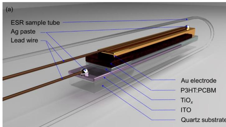
**Figure 3.** A schematic device structure of an inverted-type polymer solar cell of indium tin oxide (ITO)/ $\text{TiO}_x$ /poly(3-hexylthiophene) (P3HT):phenyl C<sub>61</sub>-butyric acid methyl ester (PCBM)/Au for electron spin resonance (ESR) measurements.
