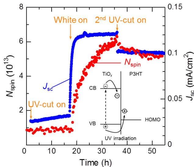
**Figure 4.** Transient response of  $N_{\text{spin}}$  (red circles) and  $J_{\text{sc}}$  (blue circles) of an ITO/ $\text{TiO}_x$ /P3HT:PCBM/Au cell to UV-cut and white light irradiation. Inset shows charge trapping scheme with respect to UV-light irradiation.
