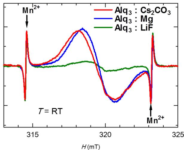
**Figure 1.** ESR spectra of  $\text{Alq}_3:\text{Cs}_2\text{CO}_3$  (red line),  $\text{Alq}_3:\text{Mg}$  (blue line), and  $\text{Alq}_3:\text{LiF}$  (green line) samples at room temperature. The spectra include those from a  $\text{Mn}^{2+}$  standard marker. Coevaporation ratio (molecular ratio) for each sample is 1:0.3, 1:0.5, and 1:10, respectively.
