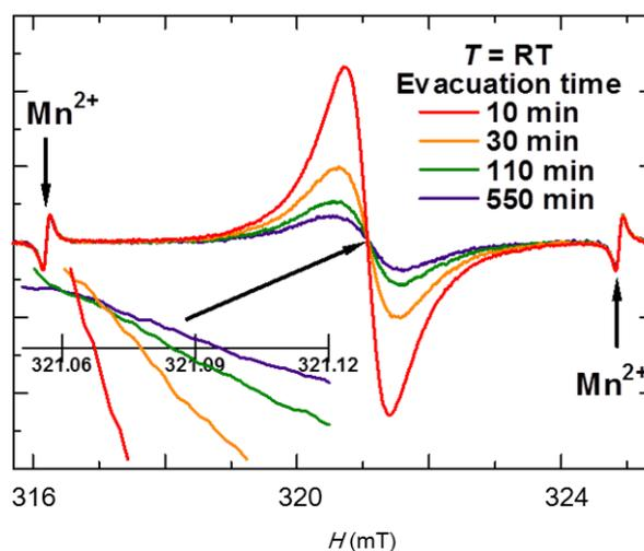
**Figure 2.** ESR spectra of iodine-doped NPB thin film with different doping concentration at room temperature. Doping concentration is controlled by evacuating the ESR sample tube. Inset shows the change of resonance center with respect to the doping concentration.
