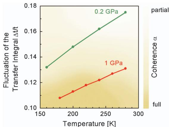
**Figure 4** Reduction of the relative thermal fluctuation  $\Delta t/t$  of the transfer integral at high pressure and low temperature. In the region of the emergence of coherent charge transport, the fluctuation is between 11 and 12%, which appears to be the critical value for pentacene.
