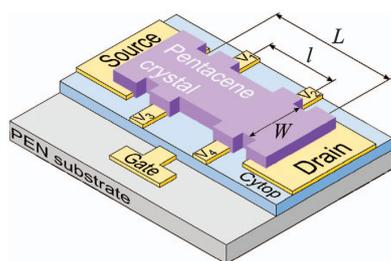
**Figure 1** Device schematics for the gated Hall measurement as well as four-terminal FET setup. First, the pentacene single crystal was placed on pre-evaporated gold electrodes, and then a Hall-bar structure was cut using laser etching. The Hall voltage and field-effect performance were measured on the same sample.
