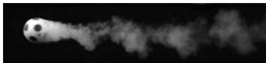
Fig. 6 Flow visualization of vortex street behind the real flight of the soccer ball (Flow is from left to right).
