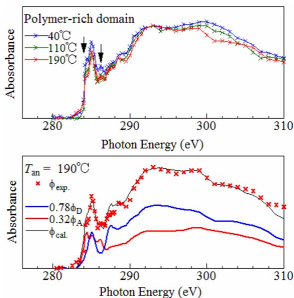
**Figure 2 | Carbon K-edge absorption spectra of the polymer matrix.** Upper panel shows the averaged absorption spectra against  $T_{an}$ . Lower panel shows an example of the spectral decomposition, which was performed by least-squares fitting of the observed spectra ( $\phi_{exp}$ ) with the linear combination of the F8T2 ( $\phi_D$ ) and PC<sub>71</sub>BM ( $\phi_A$ ) spectra,  $\phi_{cal} = C_D\phi_D + C_A\phi_A$ .
