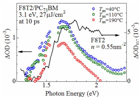
**Figure 3 | Differential absorption ( $\Delta OD$ ) spectra at 10 ps of F8T2/PC<sub>71</sub>BM blend film and differential absorption ( $\Delta OD_{EC}$ ) spectrum of electrochemically oxidized F8T2 neat film.** In  $\Delta OD$ , the excitation photon energy and pulse energy are 3.1 eV and 27  $\mu\text{J}/\text{cm}^2$ , respectively. In  $\Delta OD_{EC}$ , the hole-doping level ( $n$ ) is 0.55  $\text{nm}^{-2}$ .
