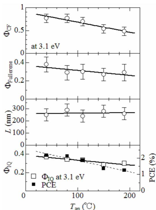
**Figure 4** | Interrelation among  $\Phi_{CF}$ ,  $\Phi_{Fullerene}$ ,  $L$ ,  $\Phi_{IQ}$ , and PCE in OSCs against  $T_{an}$ . Solid straight lines are the results of the least-squares fittings. Error bars of  $\Phi_{IQ}$  and PCE are within the symbol size.
