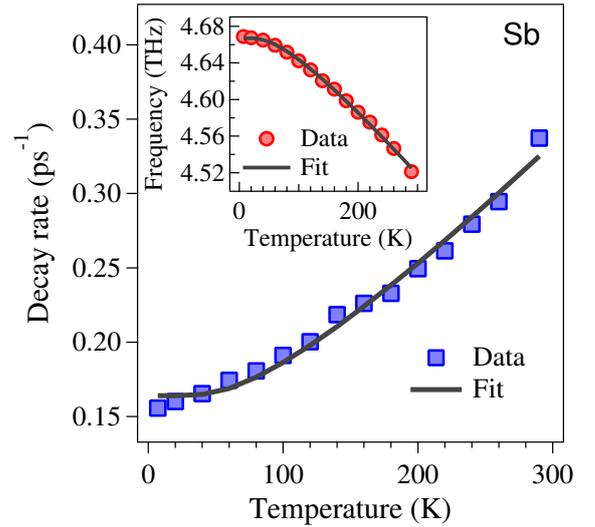
**Fig. 2.** (Color online) Decay rate of the  $A_{1g}$  mode together with frequency (inset) as a function of lattice temperature. The solid line represents the fit to the data using Eq. (2) with  $\Gamma_0 = 0.1 \text{ ps}^{-1}$  and  $\Gamma = 0.06 \text{ ps}^{-1}$ . In the inset, the frequency of the  $A_{1g}$  mode is fit to the model given by Eqs. (3) and (4), which is represented by the solid line.
