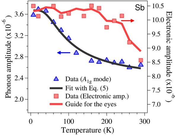
**Fig. 3.** (Color online) Amplitudes of the coherent  $A_{1g}$  mode ( $A$ ) and electronic component ( $B$ ) as functions of lattice temperature. The black solid curve represents the fit to the data using Eq. (5), using a fitting parameter of  $A_0 = 1.8 \times 10^{-6}$  and a temperature-independent background of  $1.9 \times 10^{-6}$ . The red solid line is a guide for the eyes.
