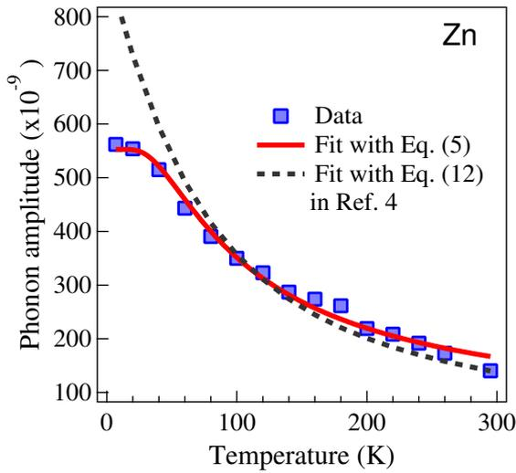
**Fig. 4.** (Color online) Amplitude of the coherent  $E_g$  mode in Zn as a function of lattice temperature (the data were reproduced from Ref. 4). The red solid line represents the fit to the data using Eq. (5), while the dashed line is the fit with Eq. (12) in Ref. 4.
