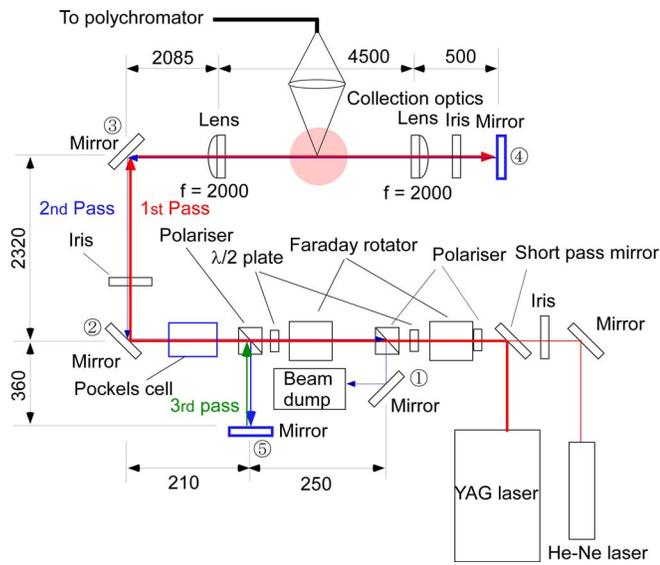
FIG. 1. Schematic of the multi-pass TS system.
