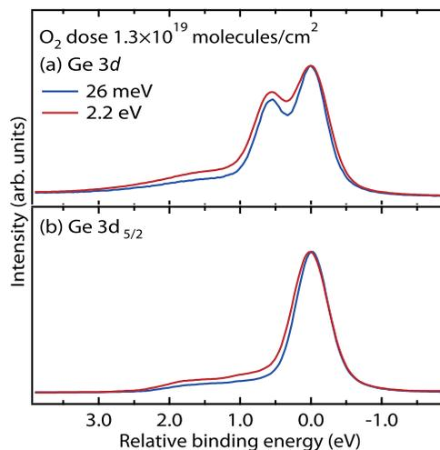
FIG. 4. (a) Comparison of Ge 3d core-level photoelectron spectra of the oxygen-saturated surface for oxygen with  $E_t$  of 26 meV and 2.2 eV. (b) Ge  $3d_{5/2}$  core-level photoelectron spectra after the subtraction of the  $3d_{3/2}$  component from (a) through the de-convolution process. The signal intensities were normalized by the Ge  $3d_{5/2}$  bulk peak intensity. The horizontal axis shows the relative binding energy with respect to the Ge  $3d_{5/2}$  bulk peak position.
