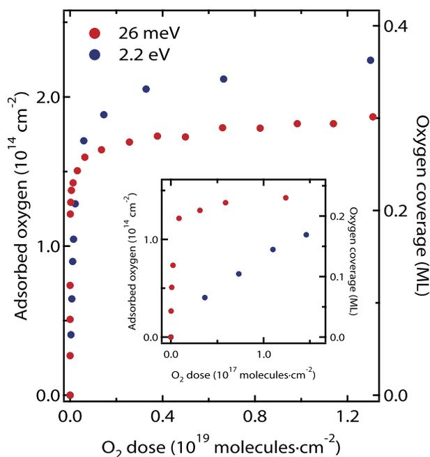
FIG. 1. Oxygen uptake curves of Ge(100)-2 × 1 surface oxidation at 300 K by thermal-O<sub>2</sub> ( $E_i = 26$  meV) and supersonic O<sub>2</sub> beams ( $E_i = 2.2$  eV). The inset shows the enlarged plots of the uptake curves to highlight the early stage of oxidation.
