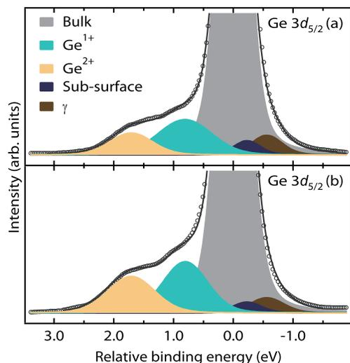
FIG. 5. Curve-fitting analysis of Ge  $3d_{5/2}$  spectra at saturated oxidation for the Ge(100) surface dosed with  $1.3 \times 10^{19}$  molecules  $\text{cm}^{-2}$  for  $E_i$  values of (a) 26 meV and (b) 2.2 eV.
