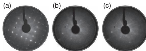
FIG. 2. Low-energy electron diffraction (LEED) images: (a) before oxidation and after saturated oxidation of the Ge(100)-2 × 1 surface at 300 K by (b) thermal-O<sub>2</sub> ( $E_i = 26$  meV) and (c) supersonic O<sub>2</sub> beams ( $E_i = 2.2$  eV).
