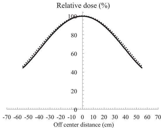
FIG. 6. In plane OCRs for  $SSD_a$  of 170 cm and  $SSD_b$  of 180 cm. Solid line and dashed line indicates the use of compensating filter at  $SSD$ s of 170 cm and 180 cm, respectively. The minus shows Gantry direction, and the plus shows a couch direction.
