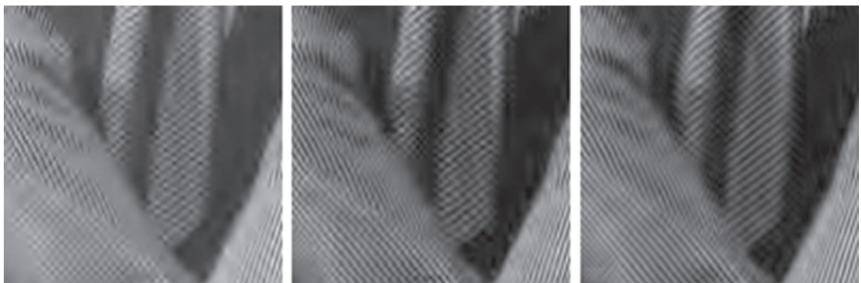
Figure 4 Comparison of particular area of reconstructed image Barbara when bit rate is 0.25 (bpp). (Left to right) 9/7-DWT, LiftLT, and 16 × 32 FLBT.
